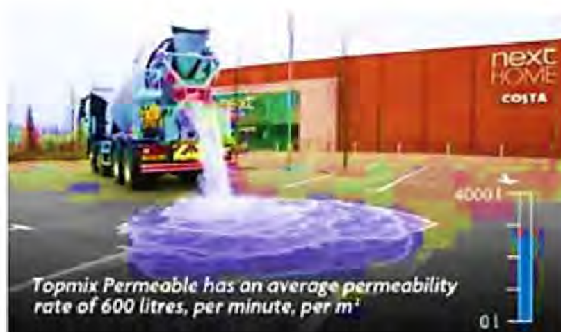
Self-drainage concrete permeability test
